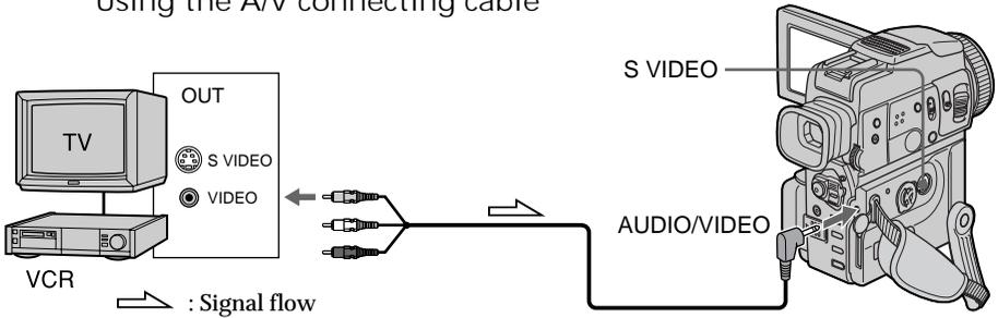
Connect the yellow plug of the A/V connecting cable to the video jack on the VCR or the TV.
