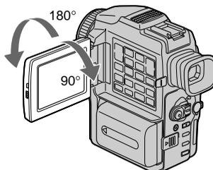
When closing the LCD panel, set it vertically, and swing it into the camcorder body.
